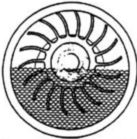
Figure 1: Water Level - Pump at Rest
